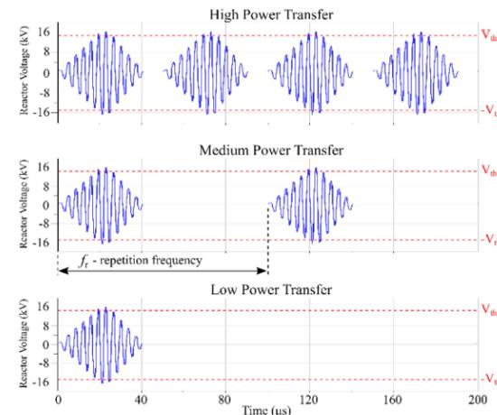
**Fig. 4.** Adjusting the active power transfer by means of varying the wavelet repetition rate.
